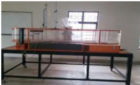
Fig. 1 Sediment circulatory loop for measurement of scour depth using graduated scale.
